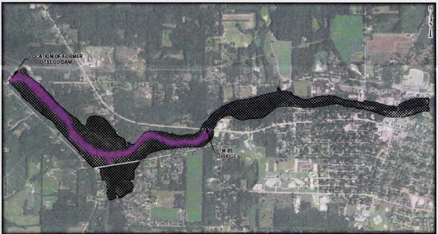
Figure showing area cleaned up by removal action upstream of former Otsego Township Dam, shaded in purple and completed in 2018. Area 3 floodplain areas evaluated for cleanup alternatives shown in grey hashing.
