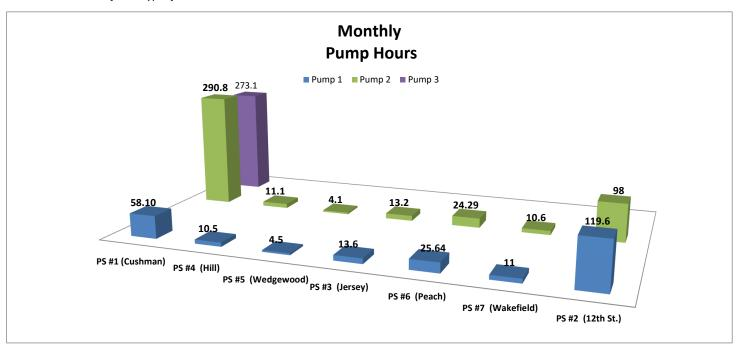
Pumps convey the waste where gravity sewers cannot, run times are a indicator of how the station is operating and being maintained.
